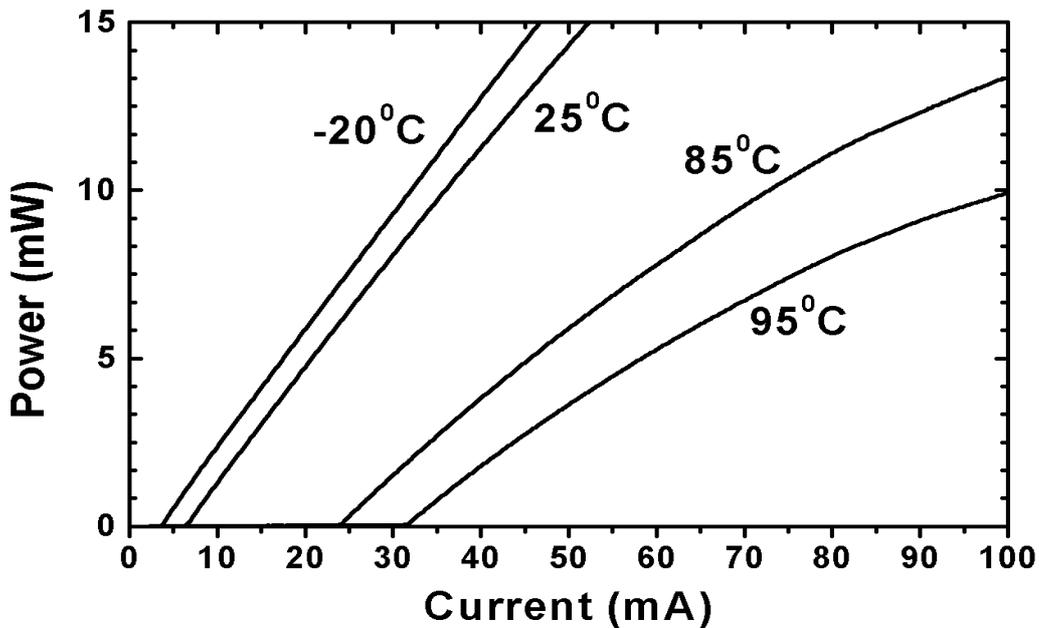
Figure 11 The variation of optical power with operating temperature. Figure used with the kind permission of Agilent Technologies
