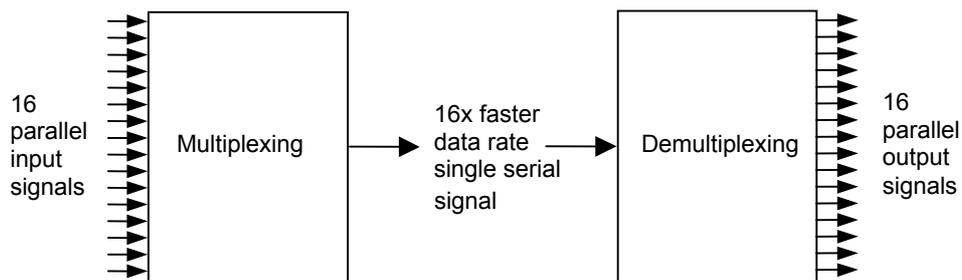
Figure 12 Schematic of time multiplexing, in this example combining 16 signals
