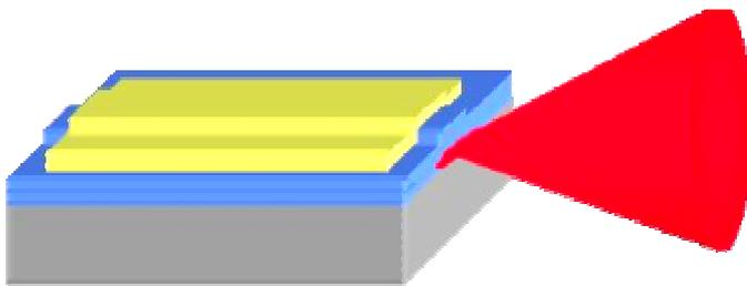
wavelengths, giving rise to a relatively broad spectral width. Because of chromatic dispersion (see page 8), the data stream at the output is smeared out. For longer distances, this design is not adequate and a different type of narrow-spectral-width edge emitter is needed, the distributed feedback (DFB) laser.
