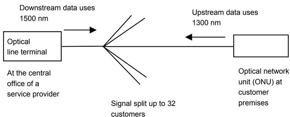
Figure 16 Schematic of a fibre system using the FSAN standard
