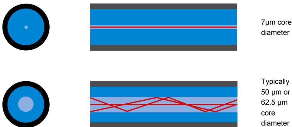
Figure 5 A single-mode and a multimode fibre (with light paths shown in red)
