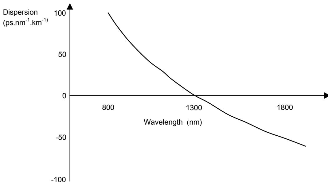
Figure 7 The variation of chromatic dispersion with wavelength
