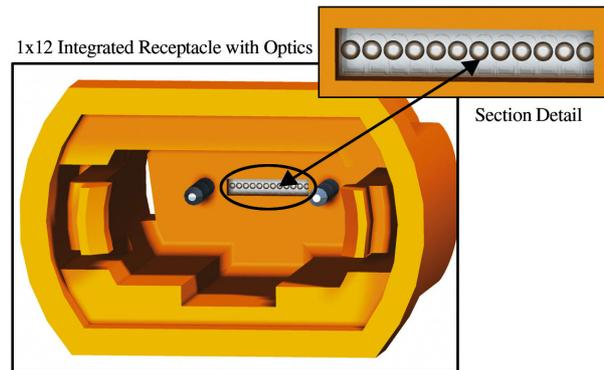
Figure 21 Lens array in a parallel optical connector (with kind permission of DOC)
