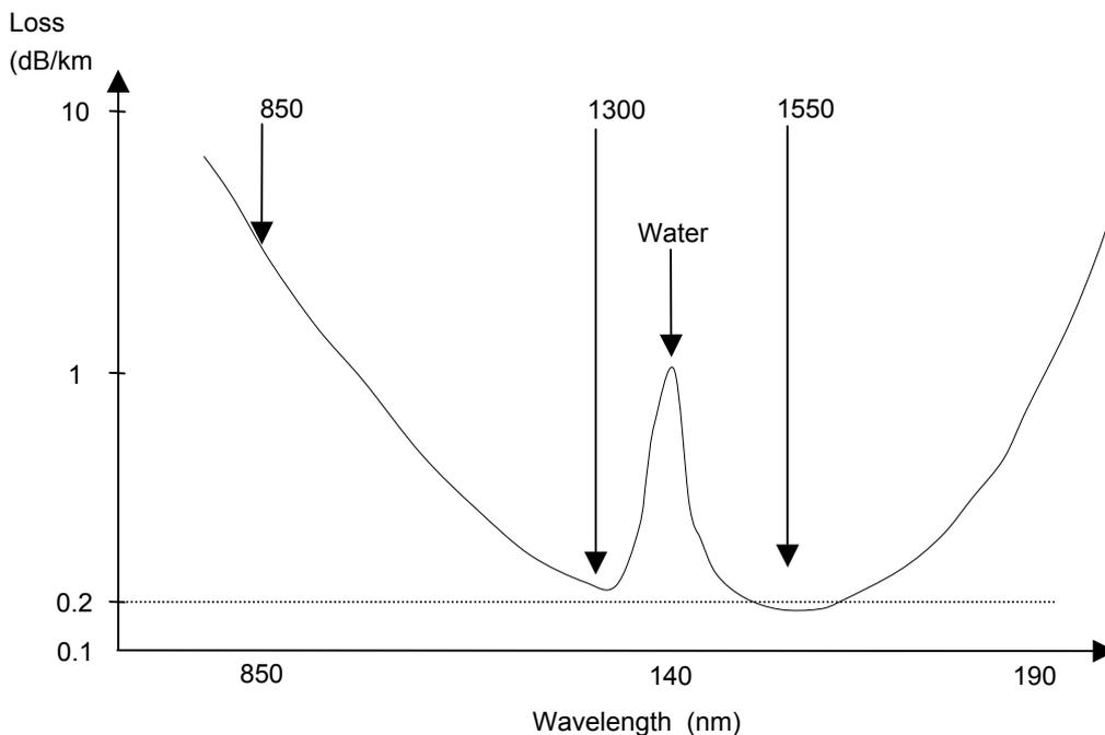
Figure 3 The variation of optical power loss with the wavelength of the light used
