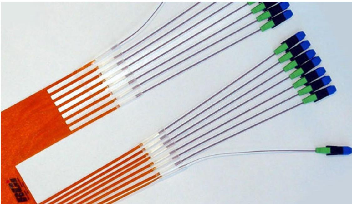
Figure 19 RCI flexfoil with ribbons and fusion splicing; connectors are MPO connectors from FCI (with kind permission of RCI<sup>43</sup> and FCI)
