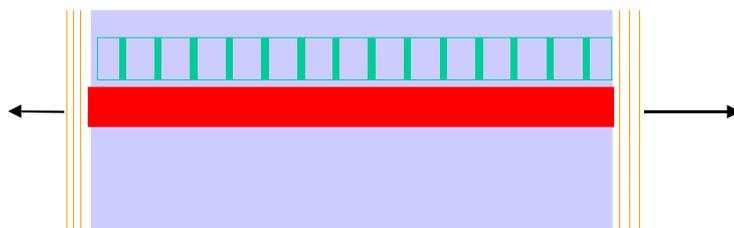
Figure 10 Schematic of a DFB edge emitter
