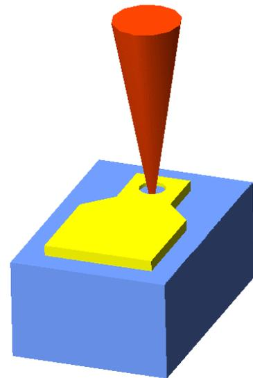
Figure 8 Schematic of a surface emitting laser
