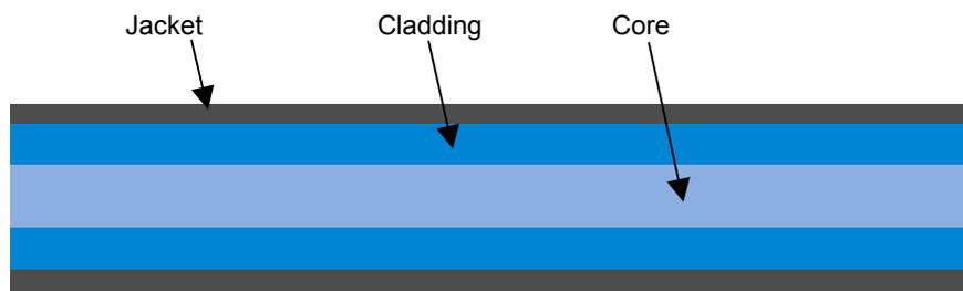
Figure 4 The structure of an optical fibre
