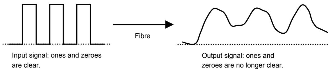
Figure 6 The distortion of data pulses due to modal dispersion in multimode fibres.
