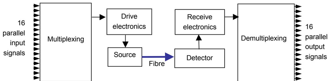
Figure 2 Block diagram schematic of an optical link
