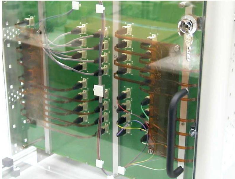
Figure 18 Optical backplane with RCI Flexfoil and connectors from FCI (with kind permission of RCI<sup>43</sup> and FCI)
