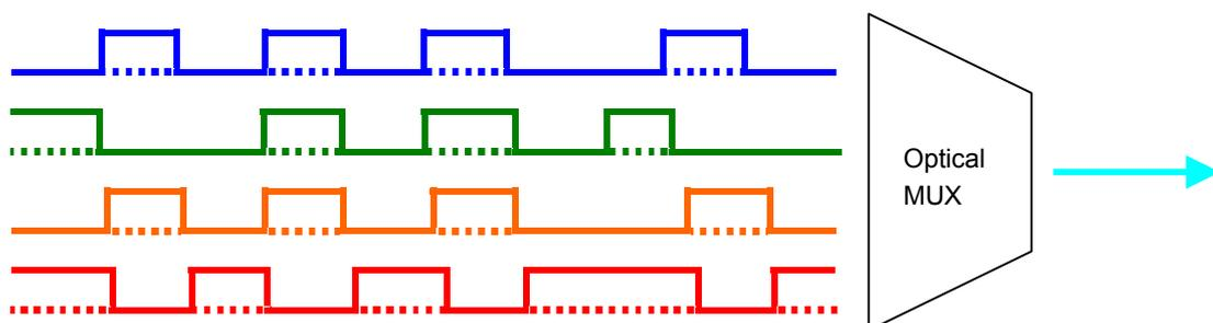
Figure 13 An optical multiplexer combines multiple signals at different wavelengths into a single multi-wavelength WDM signal
