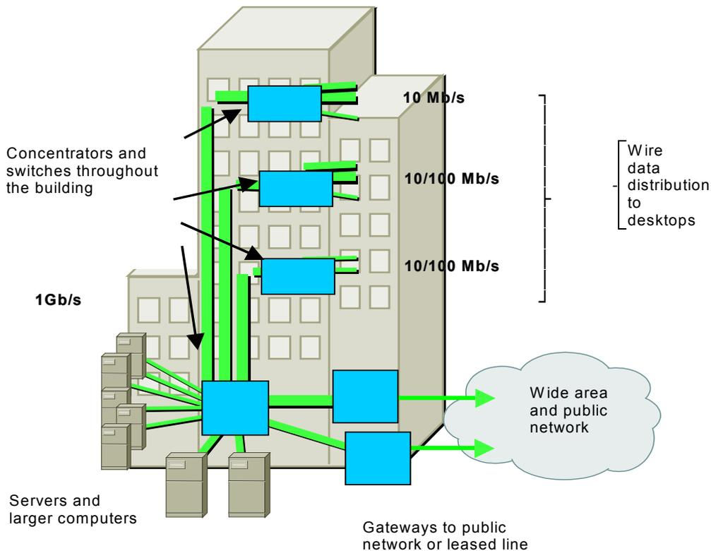
Figure 1 Data communications within a typical large building. Links carrying data above 100 Mb/s are likely to be optical.
