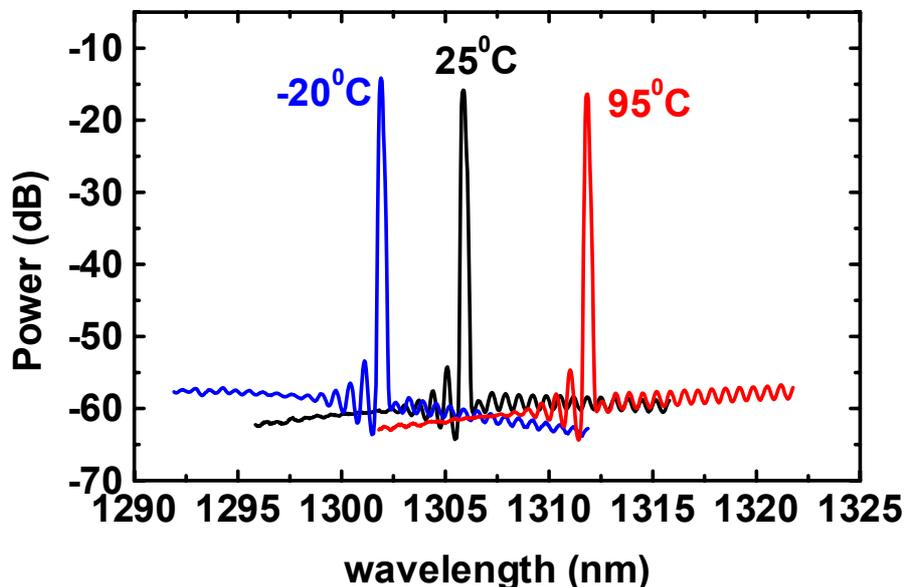
Figure 14 Inherent change of emission wavelength with laser temperature (used with the kind permission on Agilent Technologies)
