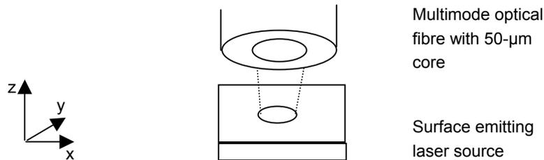
Figure 15 Optical fibre being manipulated above the laser to give the maximum optical coupling
