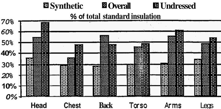
**Figure 2** This figure shows the maximum insulation reduction as a percentage of the total insulation. It occurred in the condition with maximum wind (1.0 m·sec<sup>-1</sup>) and walking speed (1.2 m·sec<sup>-1</sup>).
