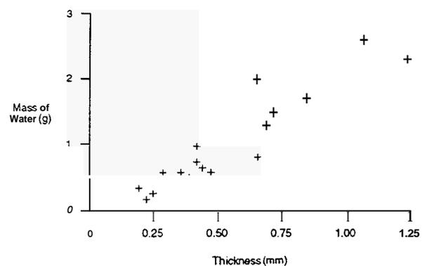
**Fig. 2** There is a good correlation between mass of water held by the fabric and its thickness. ( $r = .92$ )
