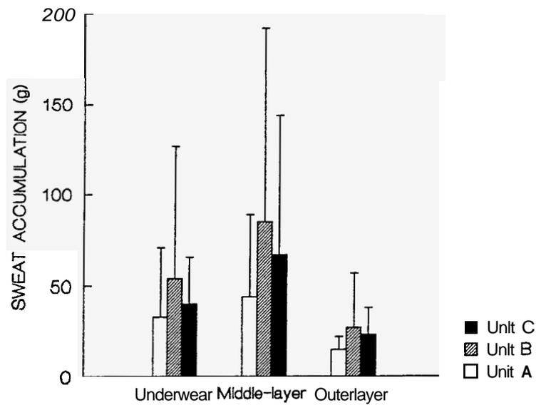
Figure 1. Sweat accumulation in underwear, middle-layer and outerlayer at an ambient temperature of +10°C (n=6).
