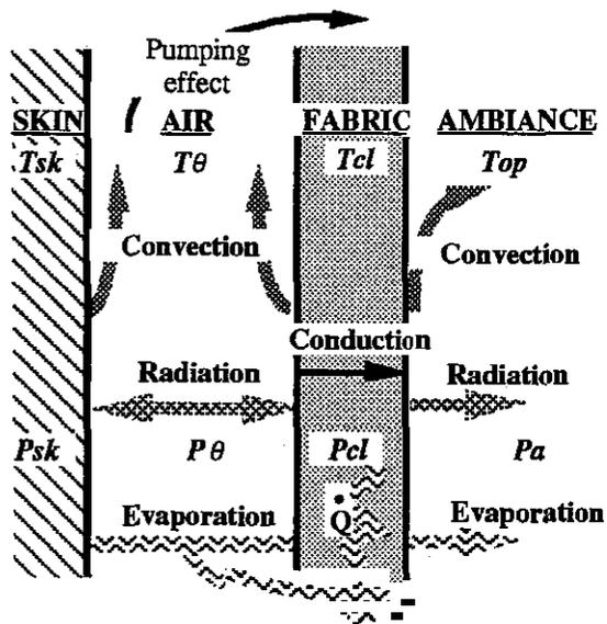
Figure 1. Representation of heat and mass transfers.
