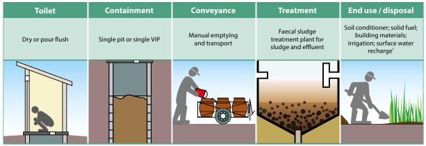
\* Sludge: treated and used as soil conditioner, solid fuel or building materials. Effluent: treated and used for irrigation or surface water recharge.
