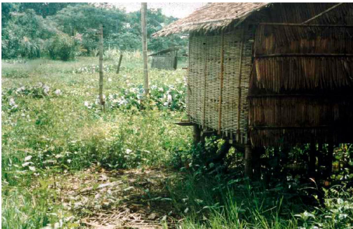
**Figure 5.** A raised latrine constructed on stilts
