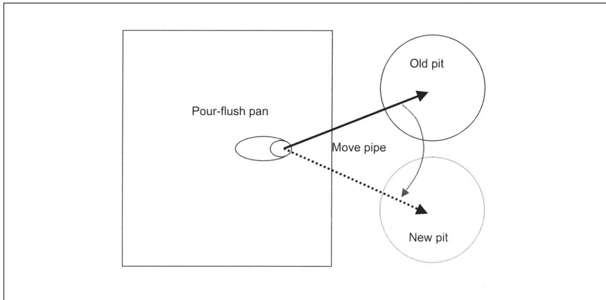
**Figure 4.** Offset pour-flush latrine with two external pits
