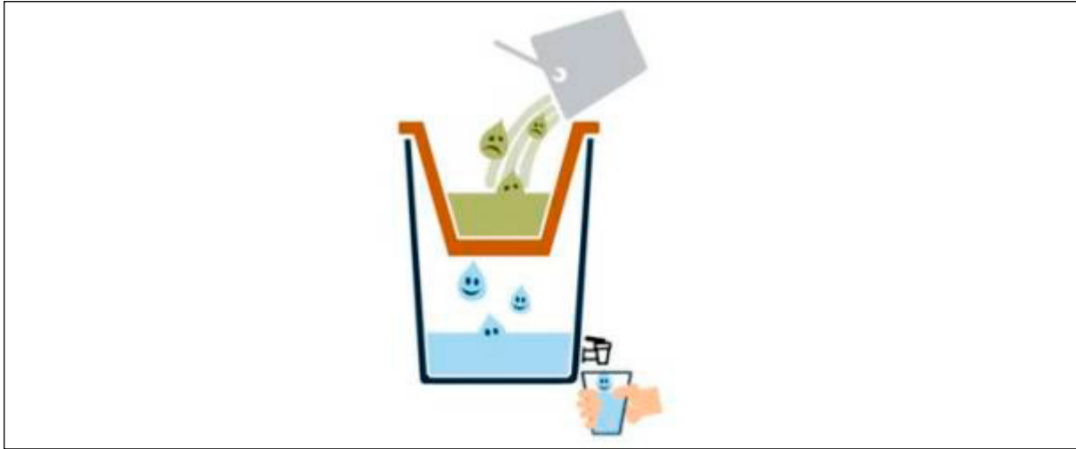
Figure 3. Figure 3: The Ceramic Silver Impregnated Filters
