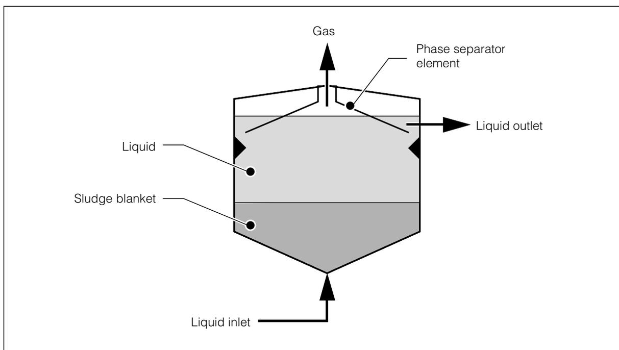
**Figure 1.** UASB digester
