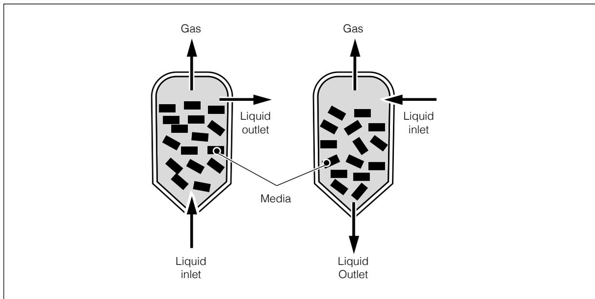
**Figure 2.** Up-flow and down-flow anaerobic filters
