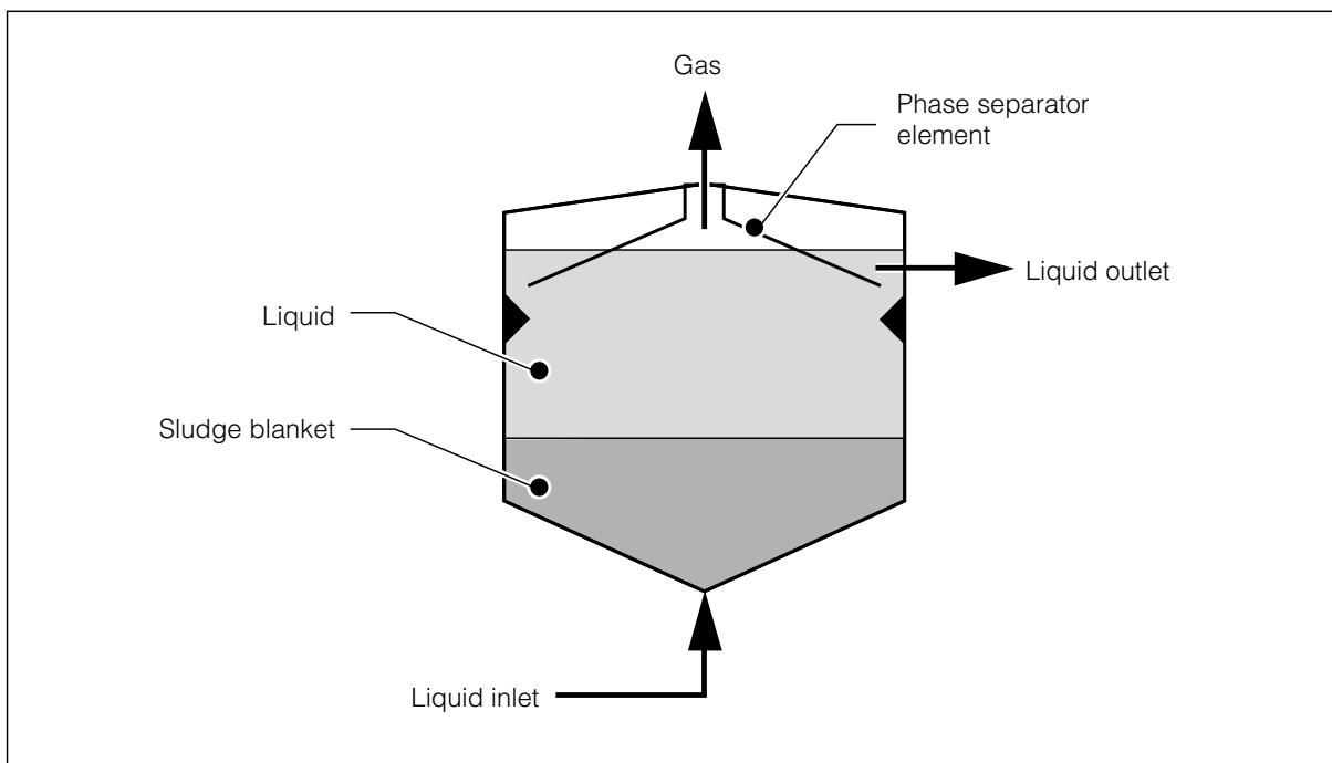
**Figure 1.** UASB digester
