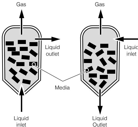
**Figure 2.** Up-flow and down-flow anaerobic filters
