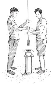
Figure 2.5. Removing the riser pipe
