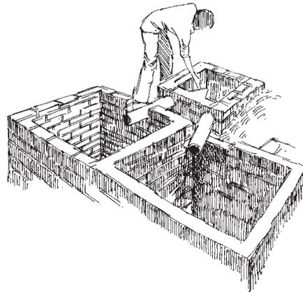
7. For public or communal latrines, for example in schools, a long pit can be divided into several chambers. These chambers are used alternately for two or three years. Each chamber receives excreta from two cubicles.
