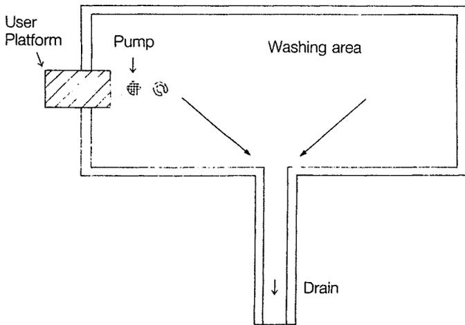
Platforms can be of all shapes and sizes as long as there is at least 600mm of impervious material around the spout. Concrete is normally used to make the surround. It is important not to over economize in the design of the slab – especially its thickness – as a cracked slab is worthless.
