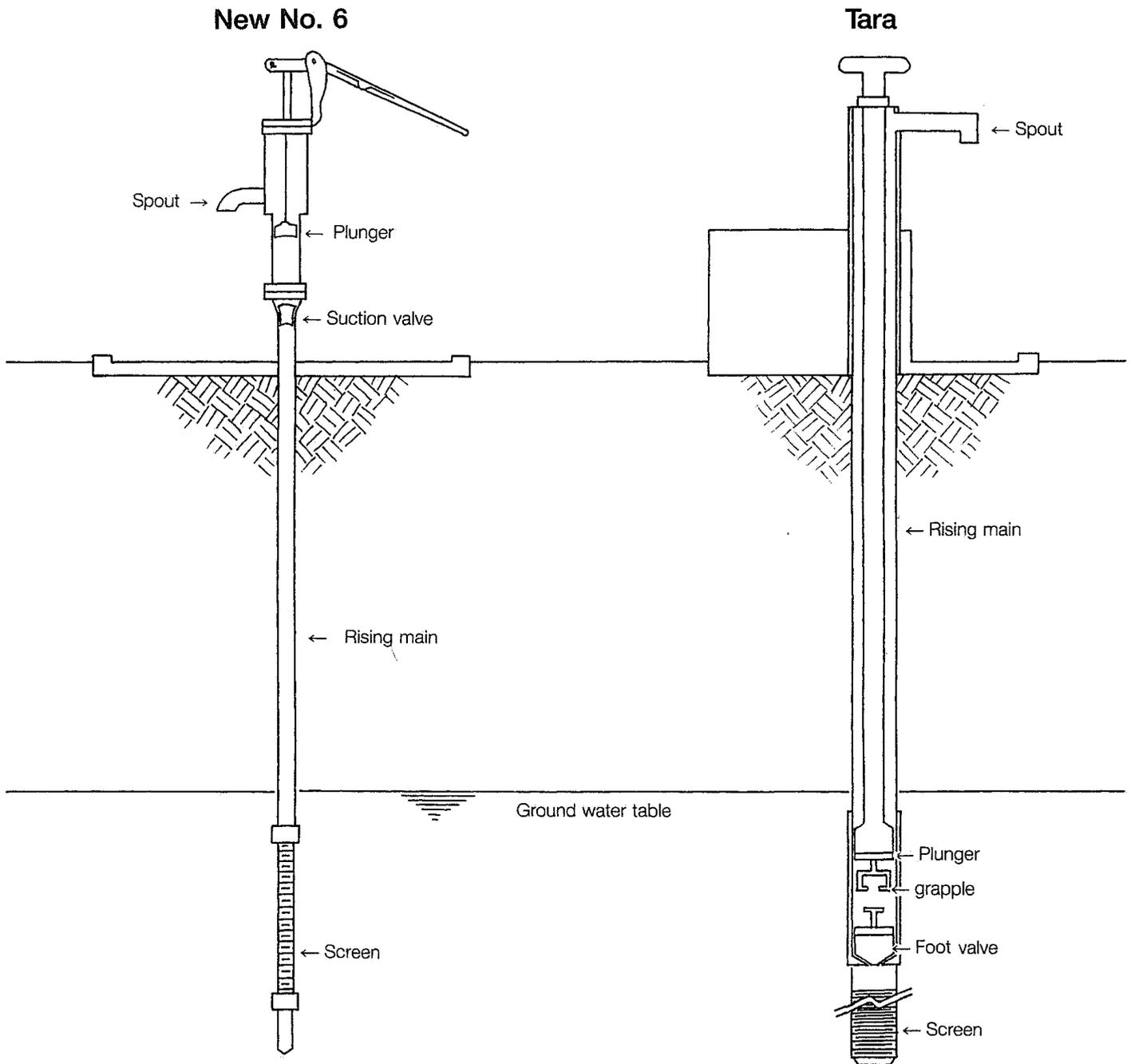
The most common form of shallow pump works by suction. The pumping mechanism is contained in the pump head above ground level. Atmospheric pressure limits maximum pumping depth to 7m at sea level (or 6m at 1,100m elevation). This form of pump requires priming to begin operation. This may mean that polluted water can be introduced into the well.
