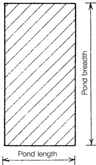
In order to ensure that the pond contents are well mixed by winds the ratio of breadth to length should be in the range 1:2 or 1:3.
