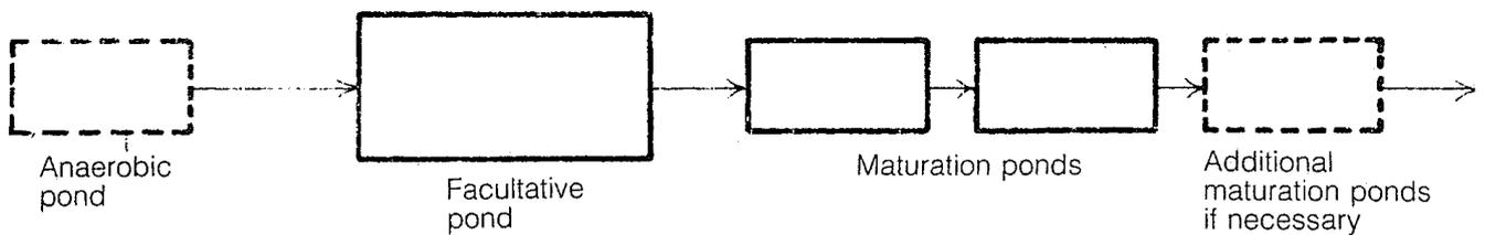
Anaerobic ponds perform the same function as septic tanks, so are not necessary if the sewage comes from septic tanks along small-bore sewers.
