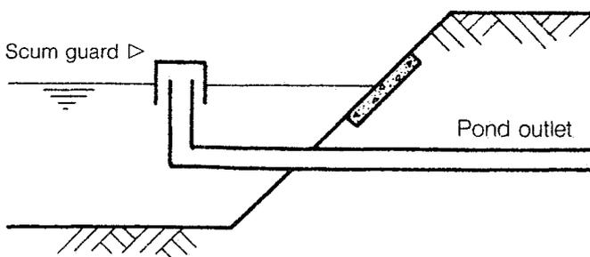
Scum guards should be provided around outlets from all ponds to prevent floating material from entering and possibly blocking the pipes.
