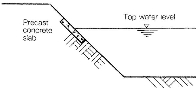
Pre-cast concrete slabs should be laid at top water level around each pond to discourage growth of weeds and to prevent bank erosion caused by wave action.
