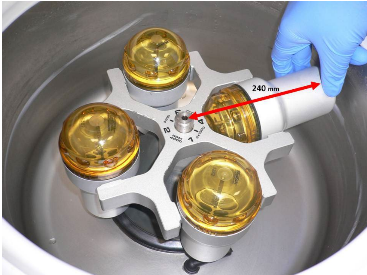
Figure 2. How to measure the radius of the centrifuge you are using: 1) Measure distance from centre to bottom of tube 2) Maximum radius of centrifuge in this example is 240 mm or 24 cm.
