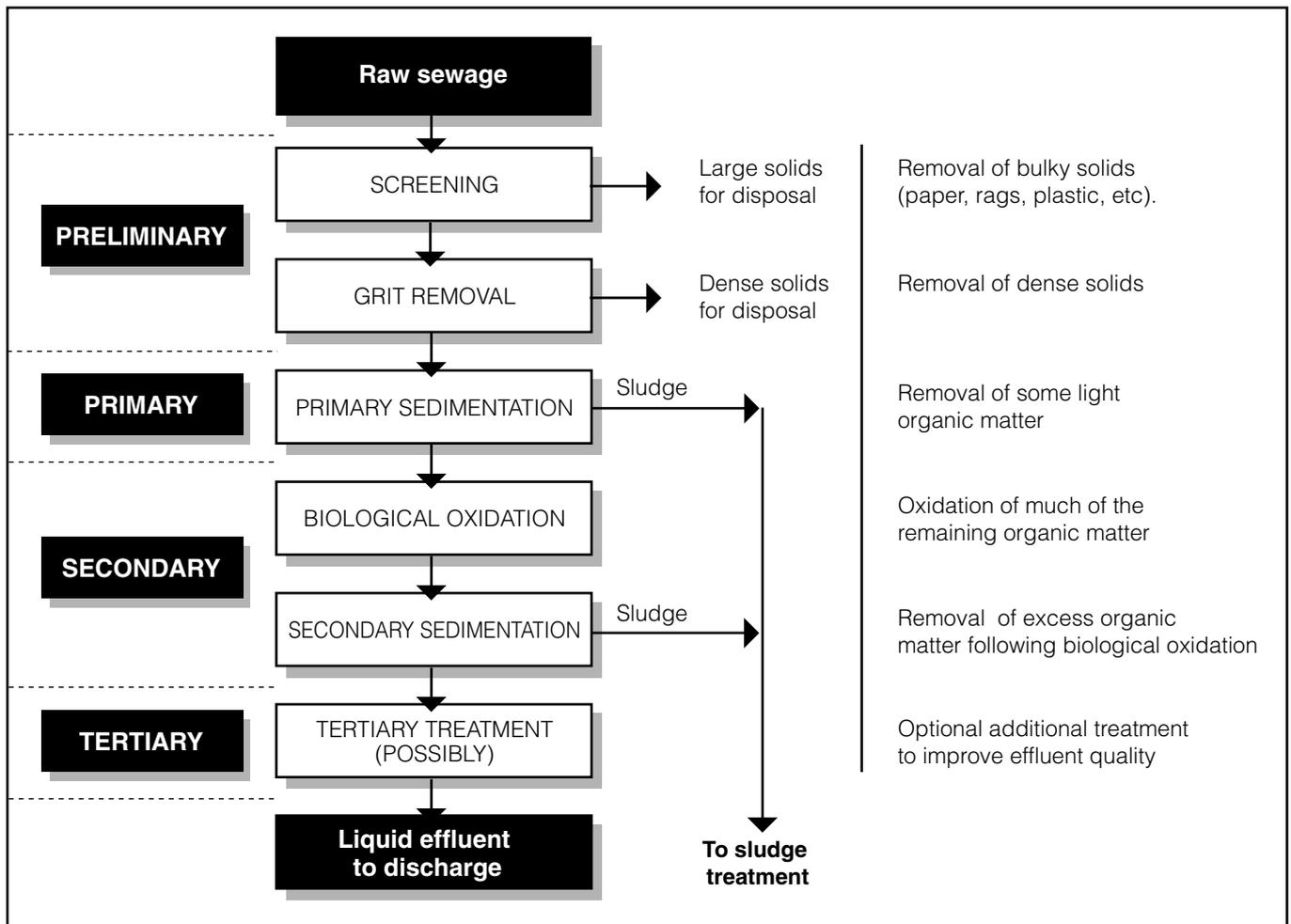
Figure 1. Typical stages in the conventional treatment of sewage
