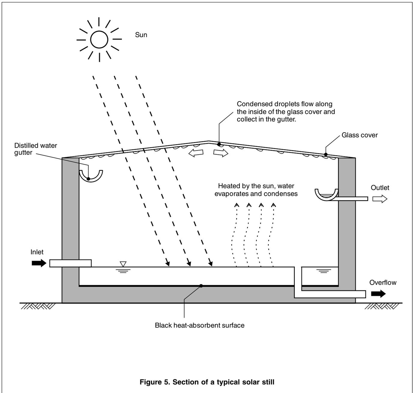
Figure 5. Section of a typical solar still
