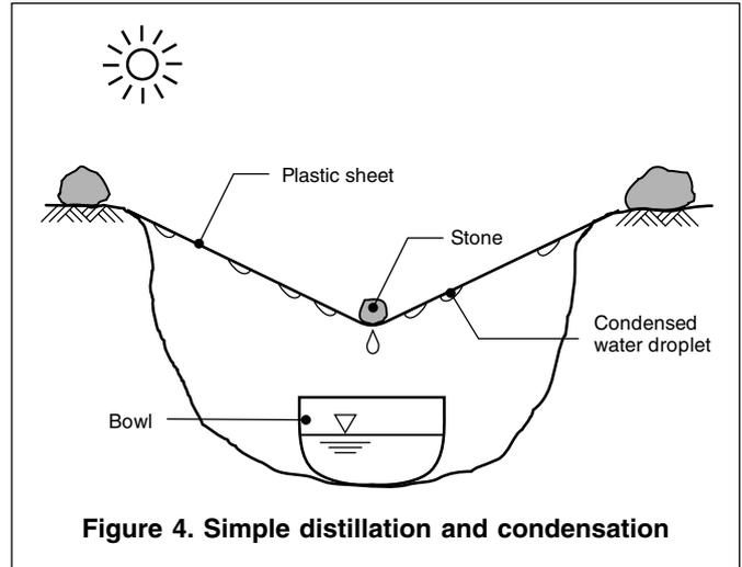
Figure 4. Simple distillation and condensation
