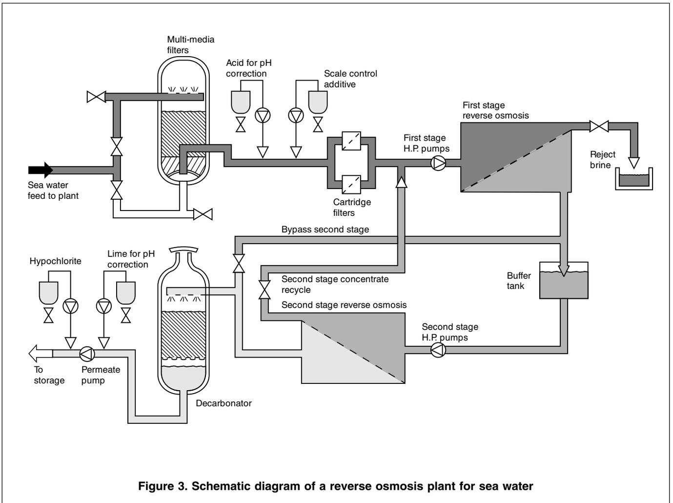
Figure 3. Schematic diagram of a reverse osmosis plant for sea water
