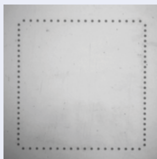
Fig 2: 75µm diameter microvia in glass and a peripheral array of microvias at 225 and 300µm pitch.
