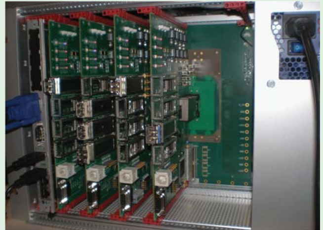
Fig. 3: 10 Gb/s Ethernet demonstrator with an optical waveguide backplane and novel 80 Gb/s aggregate self aligning optical connectors.
