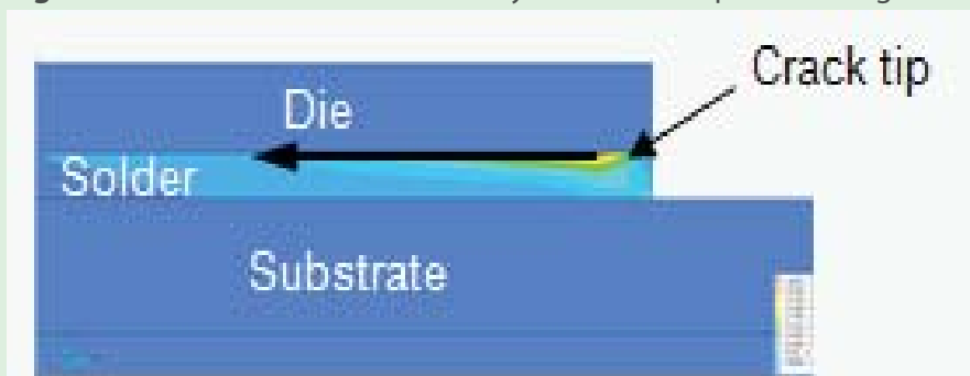
Figure 4: Modelling of the fatigue and creep behaviour of solder has facilitated development of a validated physics of failure model.
