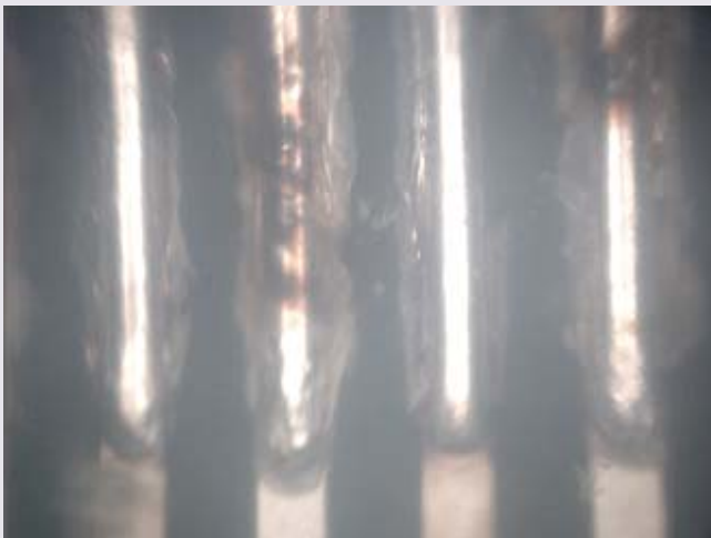
Figure 2. Discoloration on reflowed solder on bars of comb on uncleaned board after the damp heat test, seen through the encapsulation.
