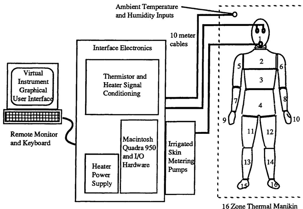
Figure 1 - Heat Pipe Thermal Manikin System
