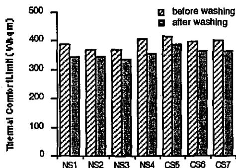
Figure 1. Thermal comfort limit of shirting fabrics
