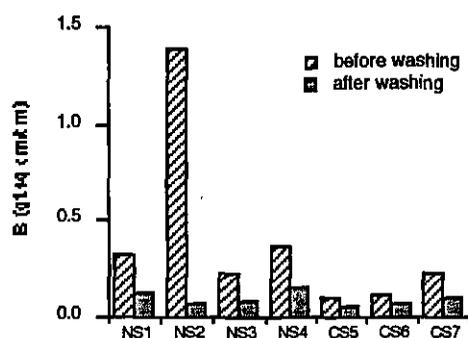
Figure 3. Bending rigidity (B) of shirting fabrics
