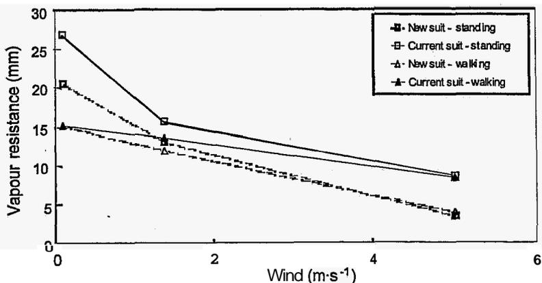
**Figure 1.** Vapour resistance (mm air equivalent) at three different wind speeds for the current suit (closed symbols) and the new NBC suit (open symbols). The data are the mean of three experiments and two sessions per experiment.
