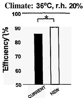
**Figure 2.** The efficiency (%) of sweat evaporation of both suits. The efficiency, defined as the ratio of evaporated sweat to the sweat produced, was significantly higher in the new suit than in the current suit (Wilcoxin signed rank sum test). The average difference was 5%
