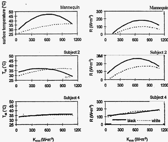
**Figure 1.** Relationships between intensity of global solar radiation ( $K_{glob}$ ) and skin temperature ( $T_{sk}$ ) as well as absorbed solar radiation ( $R$ ) in two subjects with clothing; for the comparison  $R$  values and surface temperature of a mannequin are plotted.
