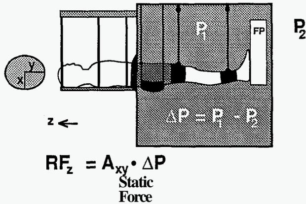
**Figure 1:** Reaction force (RF<sub>z</sub>) to generate body weight in supine posture equals the product of the cross-sectional area of the flexible waist seal (A) and the suction pressure (ΔP) as measured by a force plate (FP) within the LBNP chamber. With exercise, inertial RF<sub>z</sub>s are added to the static force.
