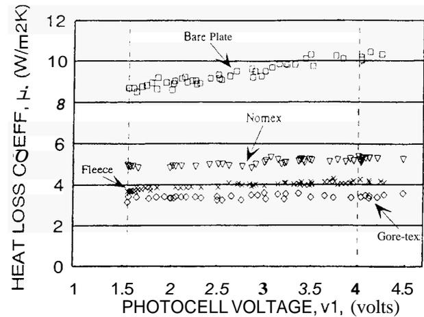
Fig. 2 - Effect of fog on fabric systems
