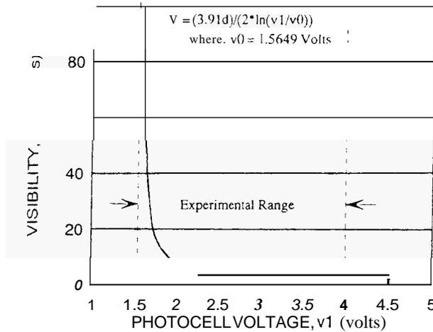
Fig. 1 - Visibility vs. photocell voltage
