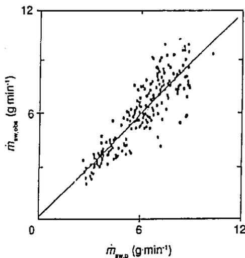
**Figure 2:** Regression between observed ( $\bar{m}_{sw,obs}$ ) and predicted ( $\bar{m}_{sw,p}$ ) mean sweat rates for experiments used for the validation of the model. I regression line  $\bar{m}_{sw,obs} = 0.84 \bar{m}_{sw,p} + 1.35$ ; II 80% confidence limit  $\bar{m}_{sw,p,cor} = 0.84 \bar{m}_{sw,p} - 0.84$
