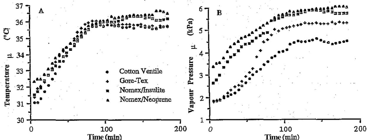
Figure 1: A) Microenvironment temperature ( $T_{\mu}$ ) and B) vapour pressure ( $VP_{\mu}$ ) within the Cotton Ventile, Gore-Tex, Nomex/Insulite and Nomex/Neoprene suits. Data are displayed at 5 minute intervals.
