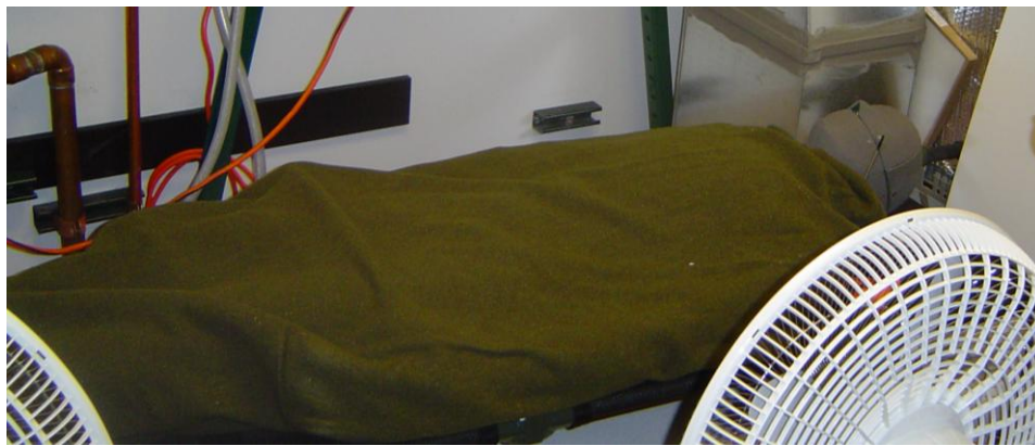
Figure 1. Test of a Wool Army Blanket Using the Thermal Manikin
