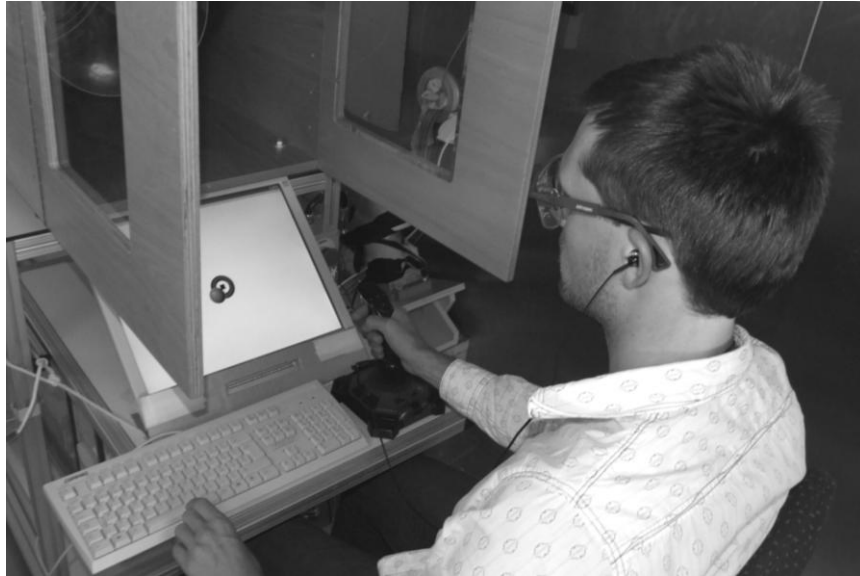
Figure 1: The first author demonstrating the simultaneous visual vigilance and tracking test (VTT) and auditory vigilance test (AVT); the screen shows the VTT.
