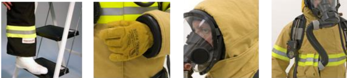
Figure 1. PFE new design features: booties, gloves, integrated hood, and hose.
