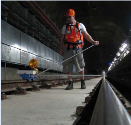
Figure1: Rail roughness measurement using the Corrugation Analysis Trolley
