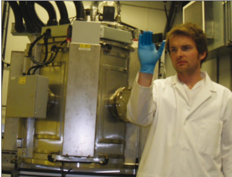
Jake Bowers inspects a thin film CdTe PV device deposited using magnetron sputtering
